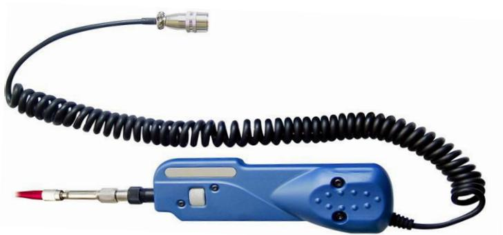
FIM-2 video microscope is used to inspect end-face of fibers and check the optic connectivity. It magnifies fibers of 125um diameter 650 times, enlarging picture through a video signal to the display where the status of fiber end-face is showed clearly in the end.
