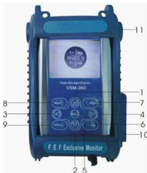
1. Up key: press when option (when observe pictures press to 5 times amplification)
